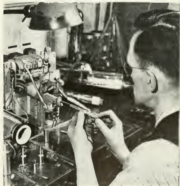
ASSEMBLING ELECTRON GUN OF CATHODE-RAY TUBES, WHICH ARE THE HEART OF RADAR UNITS WIDELY USED BY ARMED FORCES.
